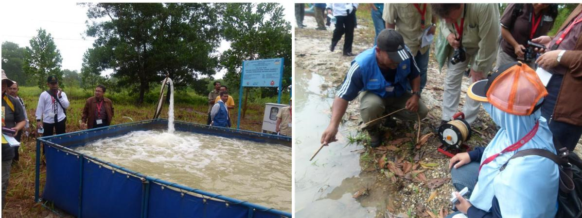
Briefing by Mr Wan Saifubahri Wan Zain from Department of Geology and Minerals. The tube well was put in by the Drainage and Irrigation Department, and managed by the Department of Geology and Minerals. The water level is checked once a week using a water level detector (pic). In dry seasons, generally from April to September, the water level is checked daily. The yield of this tube well is 70 m<sup>3</sup>
